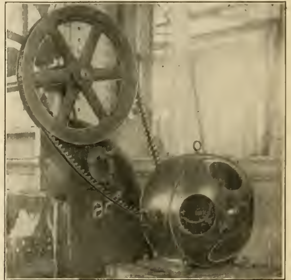
VIEW OF A CHAIN DRIVE UPON A MACHINE TOOL. RENOLD "SILENT" CHAIN.
